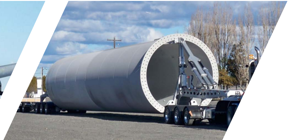
Tower Section Transporter (Schnabel trailer)
