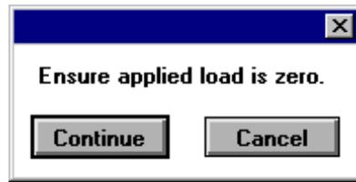
Make sure no load is applied to the load cell, then click “Continue”.
