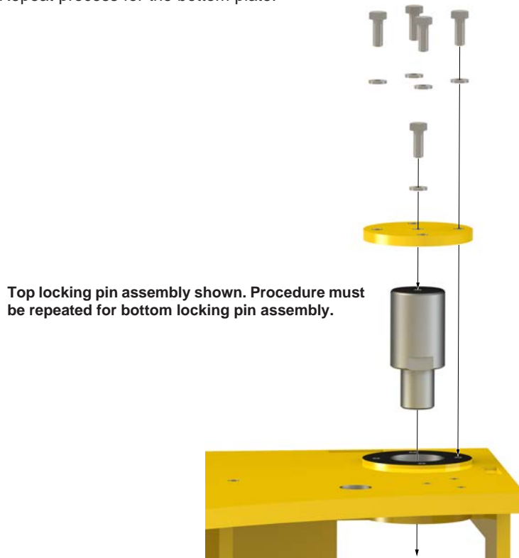
Illustration 5.9.7: Door Locking Pin Installation
