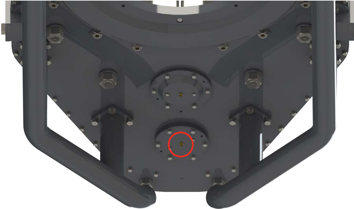
Illustration 5.5.6: Motor / Drive Lubrication
