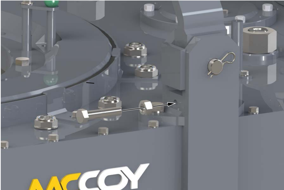
Illustration 5.9.14: Leveling Bolt Installation
