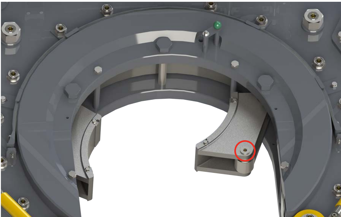
Illustration 5.5.7: Jaw Roller Lubrication
