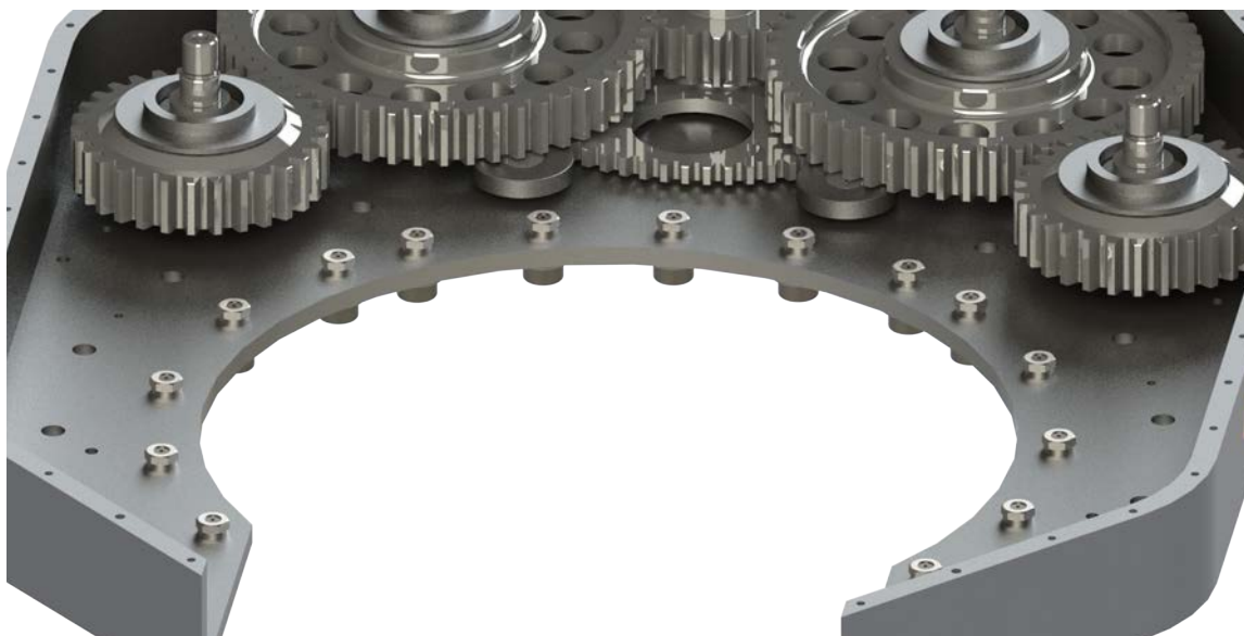
Illustration 5.9.2: Cam Follower Installation
