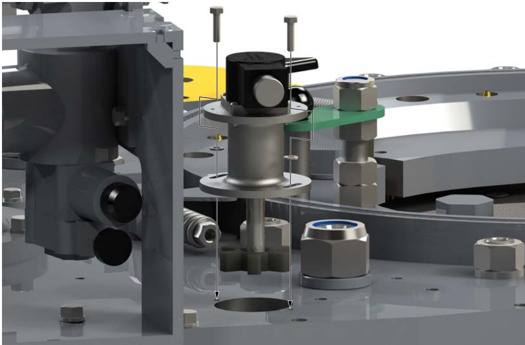
Illustration 8.1.4: Installing Encoder & Encoder Mount
