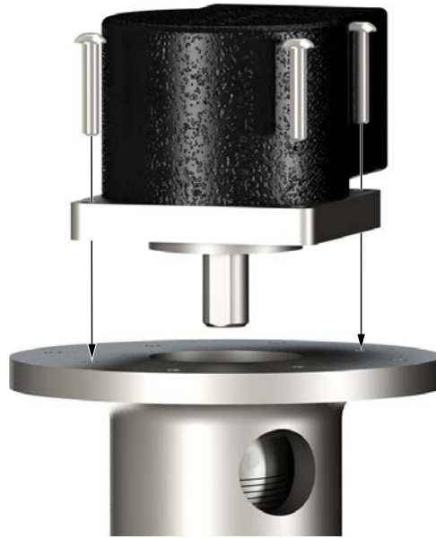
Illustration 8.1.3: Securing Encoder To Encoder Mount
