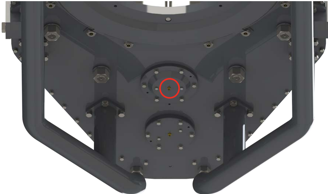
Illustration 5.5.5: Pinion Lubrication, Bottom Plate
