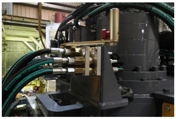
Illustration 3.3.7: Installed Control Console Pigtail
