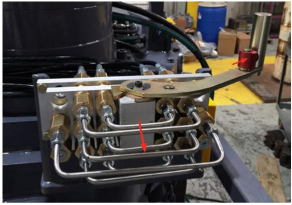
Illustration 3.3.6: Multi-connector With Installed Jumper
