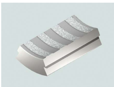
Baash-Ross® DU 5-1/2" GRITFACE® Insert Use with corrosion resistant alloy (CRA) tubulars
