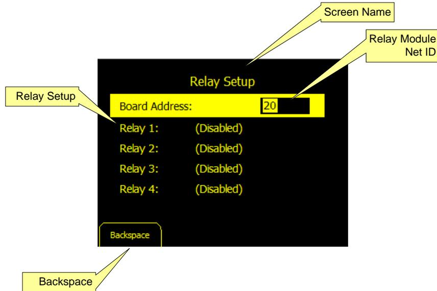
Figure 35 Relay Module Setup
